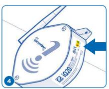
Within 2 minutes, the yellow LED should stop blinking. When the green LED illuminates, the iAquaLink is now connected.
