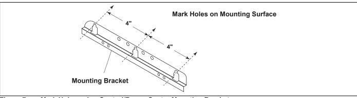
Figure 7. Mark Holes using Control/Power Center Mounting Bracket
