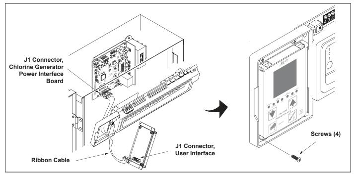
Figure 10. Installation of the User Interface
