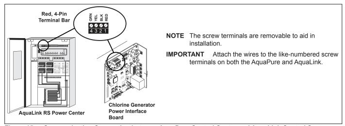
Figure 15. Communication Connection between AquaPure Control Center and AquaLink Control System
