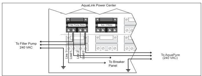
Figure 14. Power Connection between AquaPure Control Center and AquaLink Power Center
