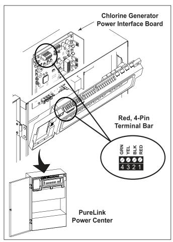
Figure 16. Wiring a PureLink Control System Network
