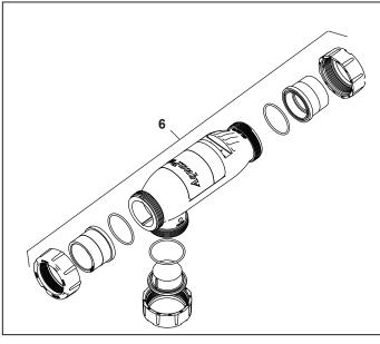
Figure 22. 3-Port Spool Exploded View
