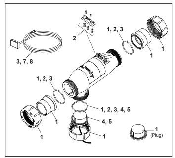
3-Port Electrolytic Cell and Sensor Figure 21. **Exploded View (Universal Unions)**
