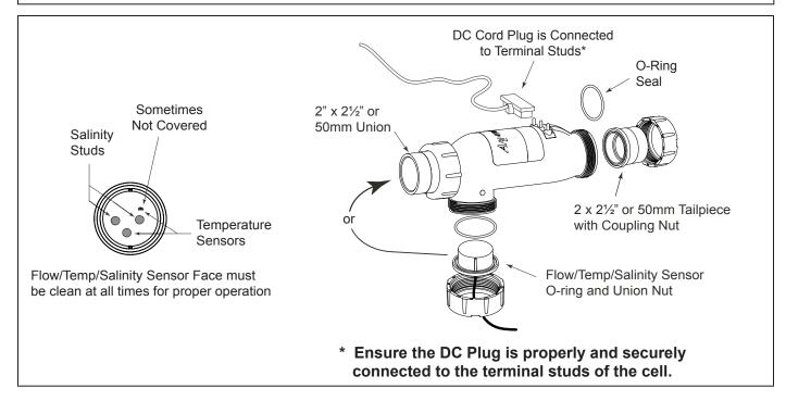
Figure 11. Cell Installation and Flow/Temp/Salinity Sensor
