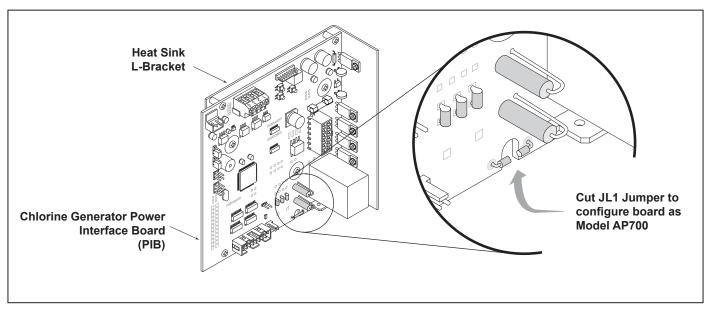
Figure 9. Chlorine Generator Power Interface Board (PIB)
