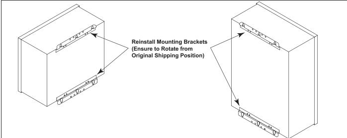
Figure 8. Reinstall Mounting Brackets on Conrol/Power Center
