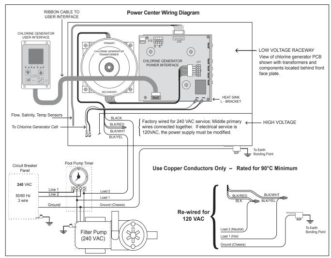
Figure 2c. Wiring Diagram for the AquaPure® System
