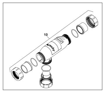
Figure 24. 3-Port Spool Exploded View
