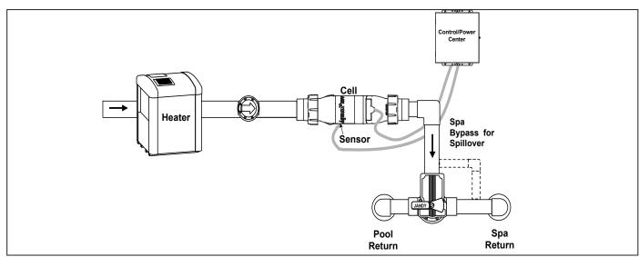
Figure 4. Recommended Plumbing Configuration for Pool/Spa Combination Systems
