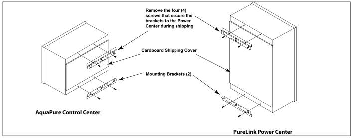
Removing the Control/Power Center Mounting Brackets from Shipping Position Figure 6.
