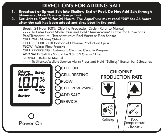
Press to increase or decrease % Chlorine Production
